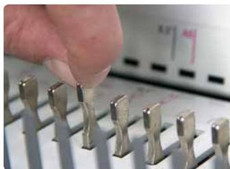
QSA (Quick Size Adjustment) technology allows the punching pins to be cancelled and the paper formats to be changed quickly and easily.
